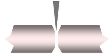
The bevel can act to guide elements that might be attached to the tube ends.
