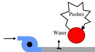
The field is the pressure field of the water in the pipe.
