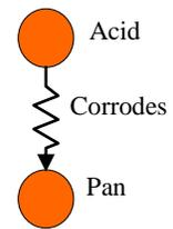
The acid performs a primary useful function in the system of corroding the coupons. The acid does not prevent, fix, make up for or counter anything. If we could have found a remedial or preventive function that it performed, perhaps we could have removed it.
