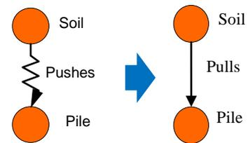
The ground must be made to perform a very unnatural act. Already, the pile is pulled down by the force of gravity. In this embodiment, it is not enough for the soil to simply move out of the way and allow gravity to perform its action. We must find a way that the soil, itself, pulls the pile into it.
