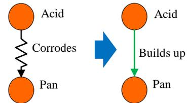
It occurs that this is a plating process which may occur if we reverse the polarity of the voltage on the pan and introduce a sacrificial material to be corroded away and deposited on the pan.
