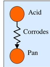
In using the full-up causal approach, we identified the harmful function of the acid corroding the pan. For the purposes of illustrating idealizing or neutralizing harmful functions, we will consider this problem through the book.
