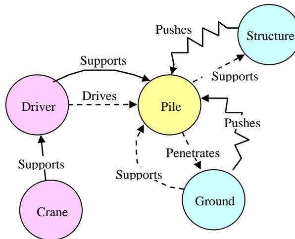
We are considering the harmful function of the ground pushing on the pile. Of course, there is an equal and opposite reaction. The pile also pushes on the ground to penetrate it. The pile actually moves the soil and the soil pushes back.
