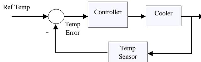
In most homes, the cooling/heating needs to be fairly accurate. A temperature sensor is added. The room temperature is fed back and compared to a reference temperature.
