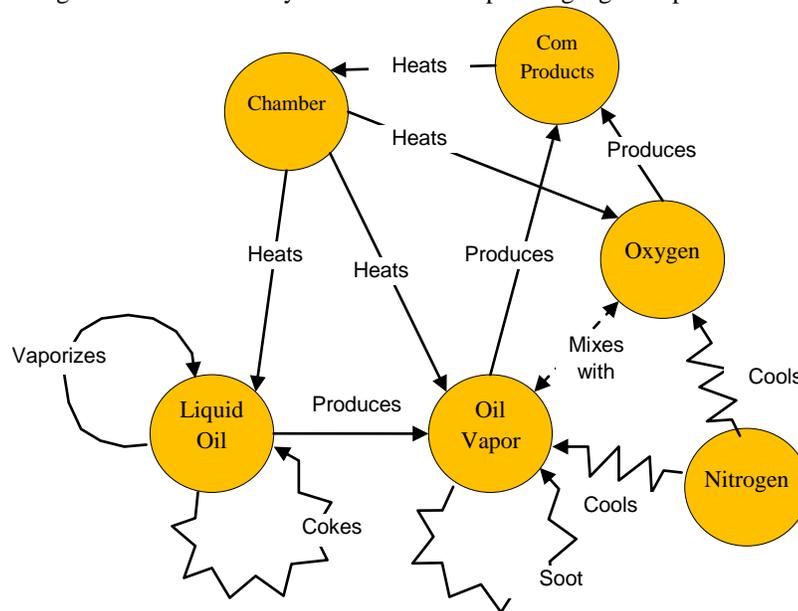
gasoline. In the case of oil, the oil must be chemically changed by the breaking of molecular bonds. The lighter species of hydrocarbon are able to be vaporized and then transported as vapor and burned. In the case of gasoline, a liquid is turned into a gas by energizing it sufficiently to become vapor. No chemical change is required. Once
